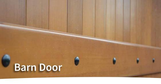
This is the Barn 86mm or 135mm door design. 86mm or 135mm VJ Western Red Cedar is fixed to a Black powder coated frame vertically with 140 x 18mm bullnose Cedar attached horizontally to the door with cup head bolts.
